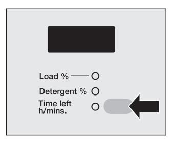
Press the button above the START button until an audible tone sounds. The sensor has now been calibrated to zero.
