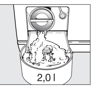
Unscrew the fluff filter lid until water runs out.
