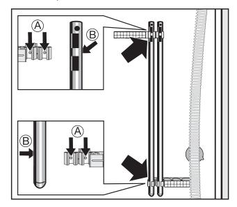
■ Secure the transit bars to the back of the washing machine. Make sure that holes **B** are fitted over retainers **A**.
